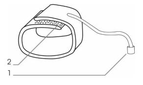
(1) Pressure connector that matches the pressure outlets on the CPAR+ Device.
