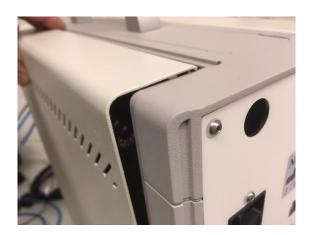
The cover can now be removed by pulling the cover forward
