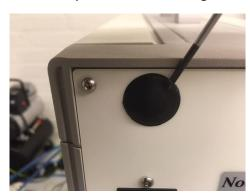
With a star screwdriver turn the screw counter clockwise
